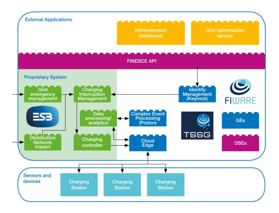
The **Distribution Impact**, provided by an external DSO system authorises the EV charging based on its knowledge of the effect that a given EV charging schedule has on the LV and MV grid conditions;
