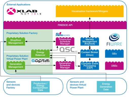
The Generation Schedule Manager DSE provides information about the VPP's energy generation. The Production Schedule Manager DSE provides the 3 production plans based on the energy requirement. The Energy Balancer takes the output of these 2 DSEs to plan how to balance the energy production and consumption. Data to identify deviations from the plan during the production is sent to the Complex Event Processing GE.
