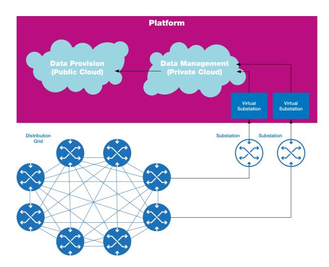
It provides all of the circuit-switched features of SDH and all of the flexibility and economics of packet-switched architectures such as MPLS. OPST supports both a distributed switched meshed topology for teleprotection applications and a centrally-switched tree topology for Energy Efficiency applications such as Load Balancing and distributed generation applications.
