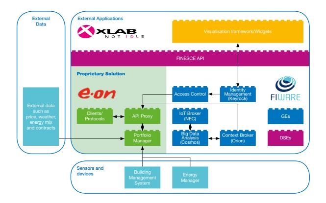
The **API Proxy** provides the external trial API and acts as a frontend integrator towards FI-Lab. As for the executing of Big Data related use cases, the **Context Broker GE (Orion)** has a very central position and interfaces to **Big Data Analysis (Cosmos). Identity Management (Keyrock)** is used for a single-sign-on to the external Visualization framework/Widgets.
